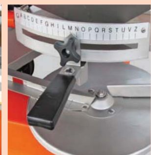
Setting gauge corresponding to the spreading charts for highly accurate fertilization
