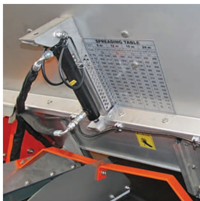
Double acting hydraulic control of fertilizer flow
